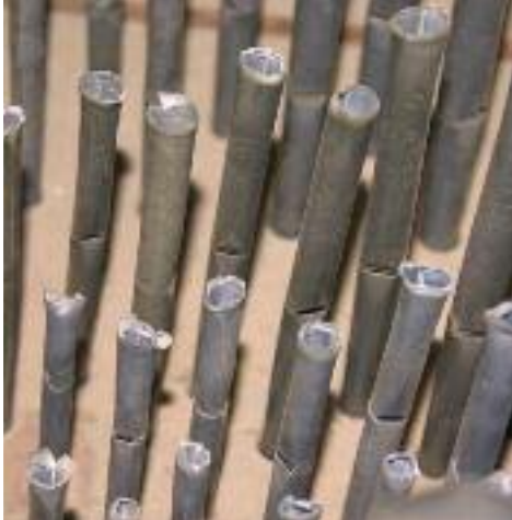
Damaged pipes in our current organ
